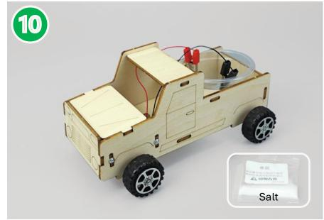
Dissolve salt with water into the clear container and insert the Carbon and Magnesium sheet into the container
